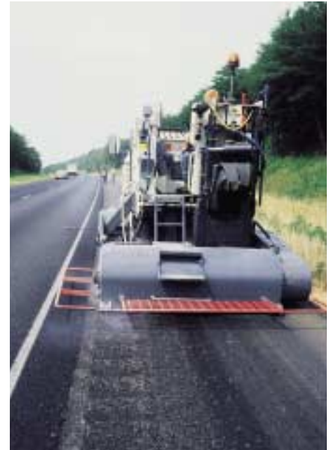
Rumble II cuts at 180 feet per minute
