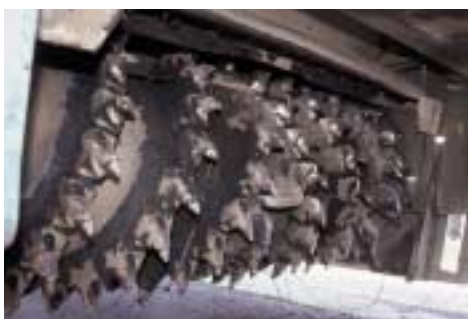
Wirtgen W 2000 unit drum is 6-foot-7 (2 meter) in width with Type III W6 teeth from Wirtgen America
