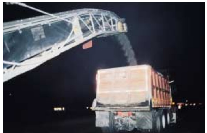
W 2200 standard cutter was working at 85 feet per minute
