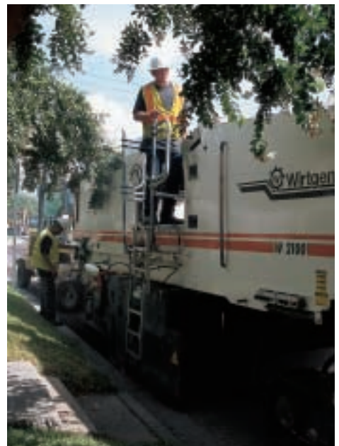
Despite its size, W 2100 mills close to curb
