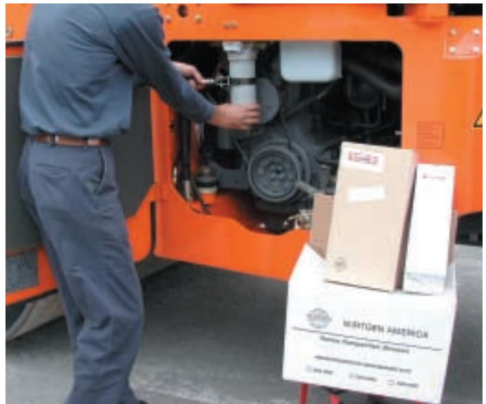
Hamm HD 130 is serviced easily using prepackaged preventive maintenance kit
